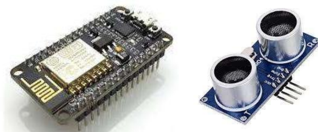
Figure 2. ESP 8266 and HC-SR04 Ultrasonic Sensor.
