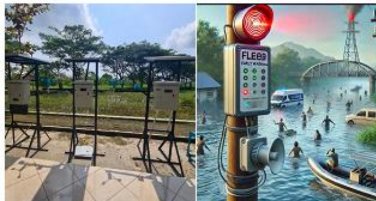
Figure 3. Example of a solar-powered flood detection device installation
