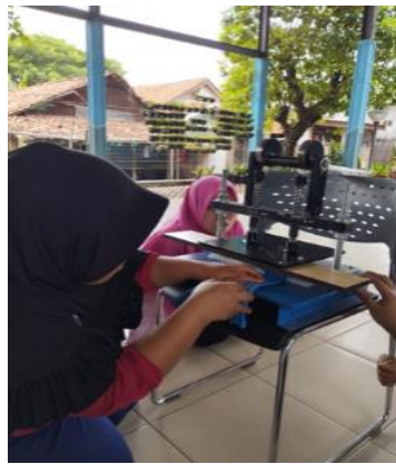
Figure 5. The clamp sheet is slipped/inserted into the bottom of the machine
