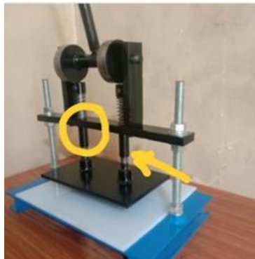
Figure 4. Sandal Clip Cutting Tool
