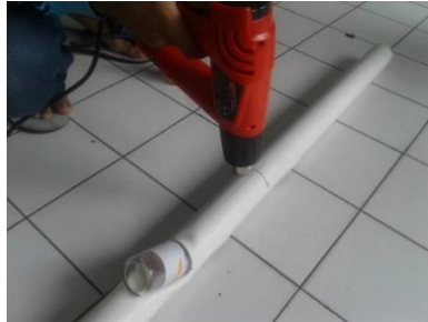
Figure 8. Heating the cut part using an acrylic heater
