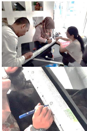
Figure 13. Making Marking or marking on paralon pipes
