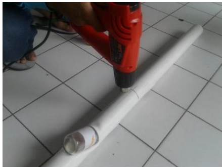
Figure 9. Making a hole using a glass bottle in the heated part
