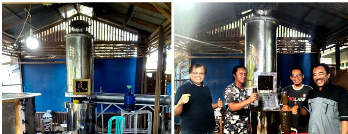
Figure 4. Testing Multi-function Equipment of Essential Oil Distiller
